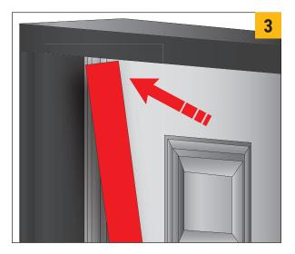
Pressing firmly, begin inserting the screw cover back into place starting at the top of the door.
