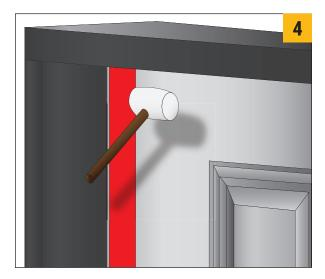
Tap the screw cover with a rubber mallet to ensure a snug fit as you work your way down.
