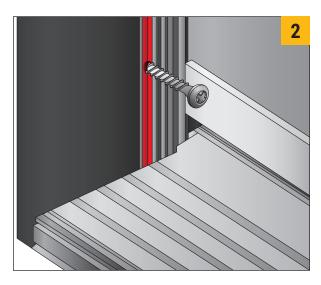
Secure the door by inserting a screw at the designated location in accordance with installation standard CSA A440 .4.
