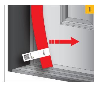
Grasping the label, pull the screw cover gently upward to remove it completely from the frame. This step does not require the use of tools.
